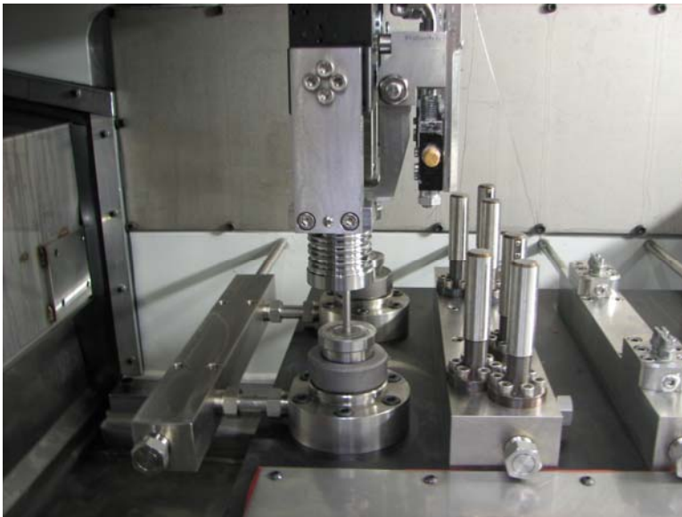
Internal part feature being deburring with a rotary lance nozzle (shown without water for clarity).
