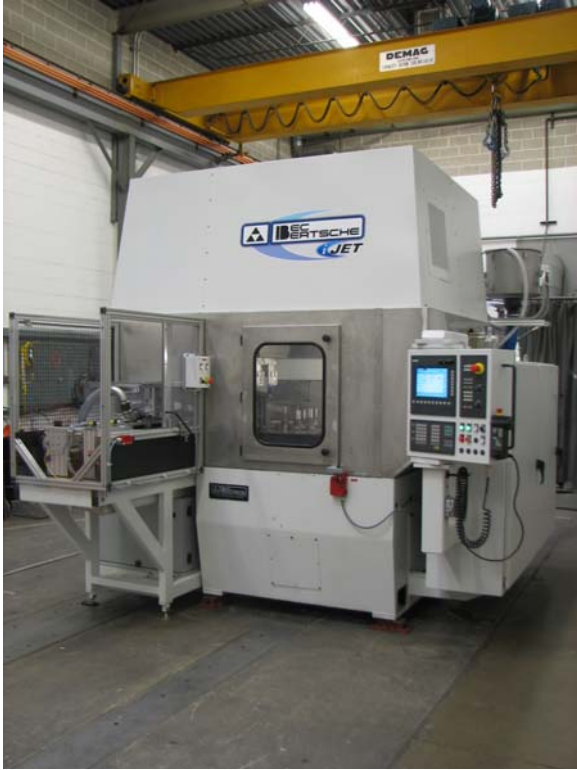
Bertsche 4 axis (X,Y,Z and C axis) i-Jet with integral drying station and post deburr part rinse station
