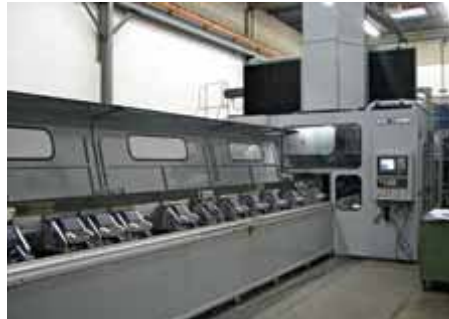
Bertsche Engineering A custom metalcutting machine tool from Bertsche Engineering.
