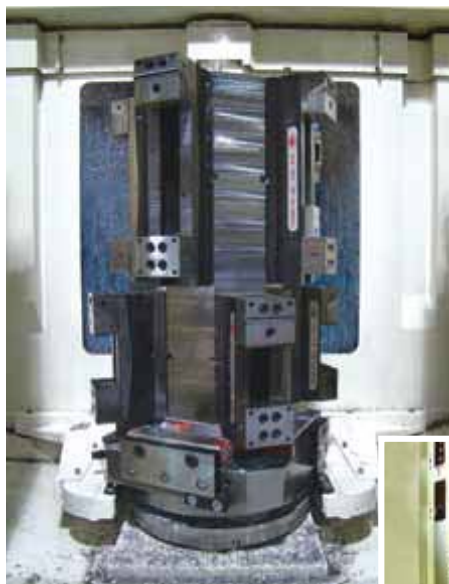
MTT-21 designed special fixtures for Schultes' Kitamura Mycenter-HX400iF HMC to provide appropriate spacing between the manually operated vises and enable adequate clearances for the array of tools applied (inset).
